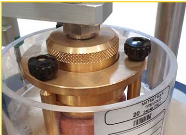
Brass oedometer cells with fixed ring, having diameters from 50.47 to 112.80 mm
