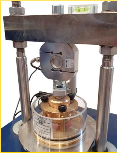
Mobile crosshead for vertical clearance adjustment and adaptation to different cells.
