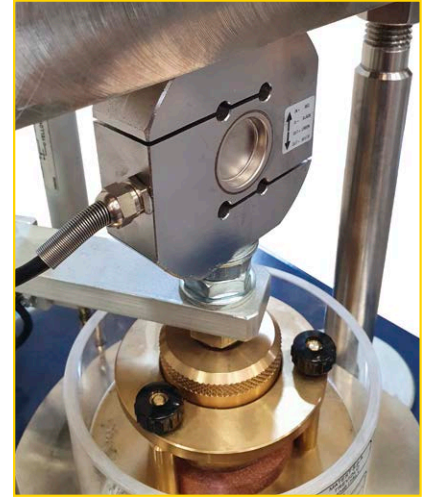
Possibility to install load cells having different capacities, in addition to 10 kN standard load cell.
