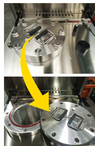
Easy to open: the cover of the vessel can be placed in a resting position easily by the operator.
