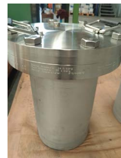
Pressure vessel is CE, PED and ASME certified to resist at a design pressure of 24.5 bar at 148 °C
