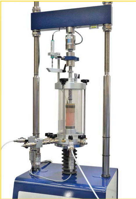
Triaxial cells to accommodate samples from 38 mm to 150 mm.
