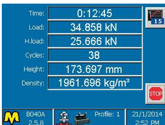
Test parameters during compaction
