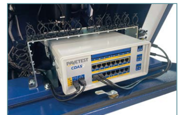
Control and Data acquisition system (CDAS2) located under the test chamber. It houses the cables and trasducers limiting the footprint of the machine and keeping the test area, tidy.
