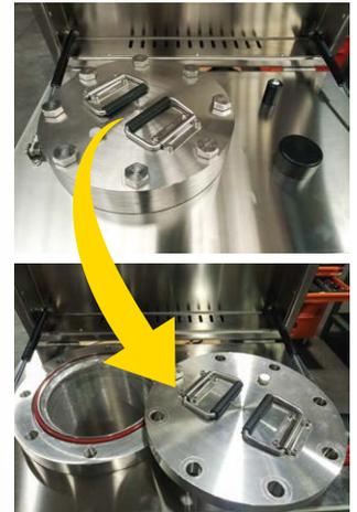
Easy to open: the cover of the vessel can be placed in a resting position easily by the operator.
