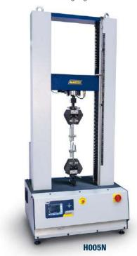
The frames protecting the columns and the screws are made of painted steel sheets, the internal sides are closed with anti-dust bellows and all the outside and internal parts are properly treated against the corrosion.
