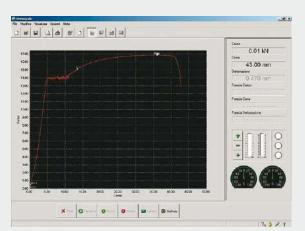
Tensile test on a steel specimen without extensometer; it displays the yield poind with the possibility of increasing the dimensions of the graph area by means of the zoom function.
