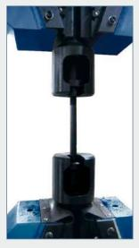
Tension on threaded and shouldered head samples
