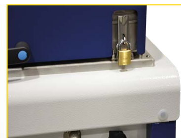
Safety lock of distillation chamber in order to avoid any accidental opening by the user.
