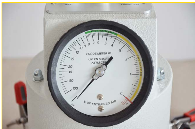
The manometer allows you to read the percentage value of air trapped in the sample.
