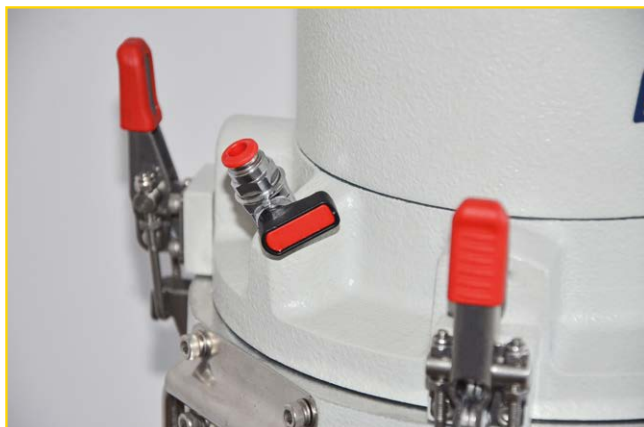
Opening-closure valves for air-water inlet and outlet.
