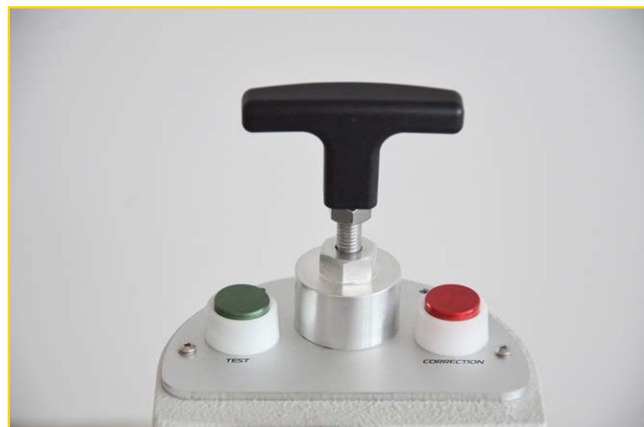
Sturdy hand pump for generating pressure into the chamber. Buttons for pressure release and precise adjustments.
