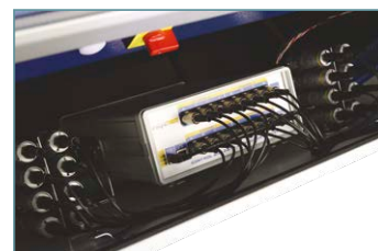
Control and Data acquisition system (CDAS) located under the test chamber. It houses the cables and trasducers limiting the footprint of the machine and keeping the test area, tidy.
