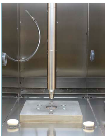
Motorized contrast shaft that is used to modify the space in the chamber according to the test and sample used.
