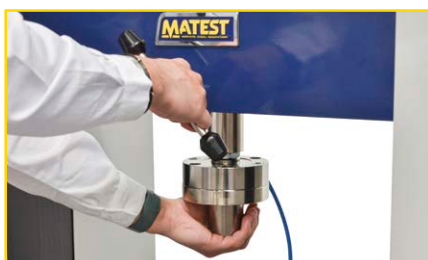
Removable pin for fast replacement of accessories
