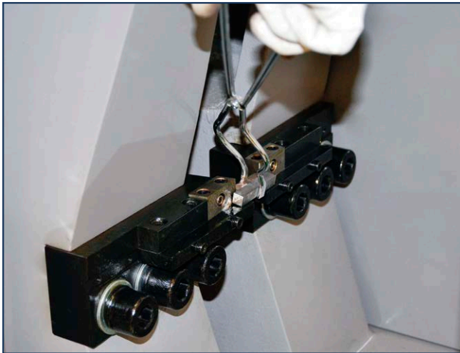
Specimen positioning on H062-01M using pliers H054
