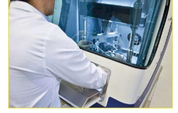
A small window offering access to the test space with minimal disruption to the chamber temperature.
