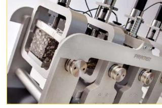
B210-01 Servo-pneumatic four point apparatus, detail
