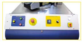
Thermoregulation display to monitor the temperature in real time.
