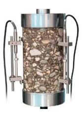
B264 KIT Direct tension testing kit
