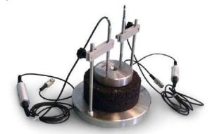
B260 KIT Uniaxial cyclic compressionComprises:B260-01NBase assemblyB260-02Chamfered top platenB290-02NLVDT (10 mm) (2 pieces)
