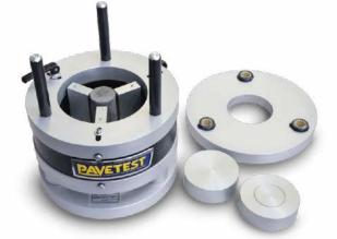
**B202** Gauge Point Fixing Jig + accessories for small specimens preparation
