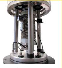
Asphalt specimen with on-specimen LVDTs and load cell
