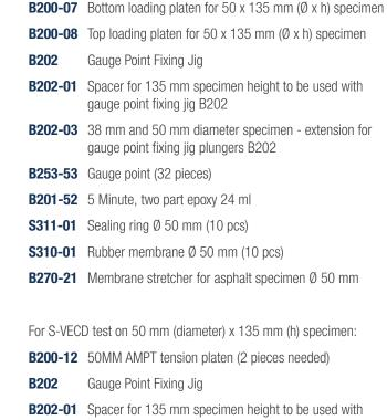
For dynamic modulus on 50 mm (diameter) x 135 mm (h) specimen:
