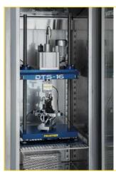
B220-02 KIT DTS-16 detail B220-12 20 kN Load frame with motorized crosshead
