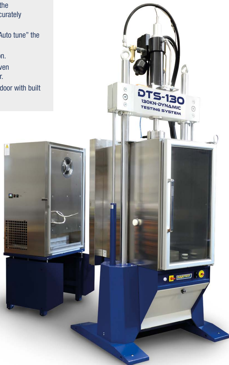
Two piece temperature controlled cabinet
