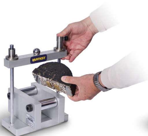
Asphalt specimen positioning
