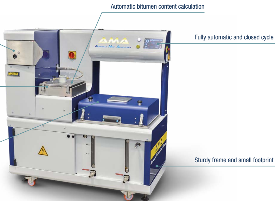
Cup into the centrifuge, up to 8000 revolutions per minute
