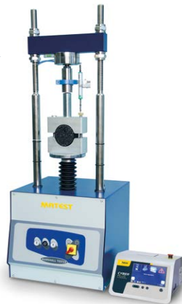
B043-KIT DIGITAL MARSHALL TESTER 50 KN CAPACITY
