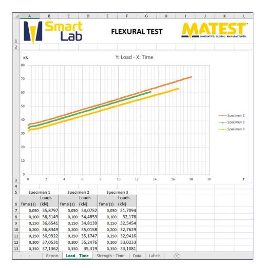
According to the relevant verification procedures for the determination of concrete quality, SmartLab allows to generate a report including different tests (up to 10) to easily compare the data.
