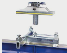
Flexural toughness (ASTM C1550)
