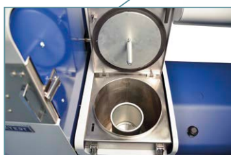
High speed centrifuge. Inspection window on the cover is used to monitor the solvent colour during extraction.
