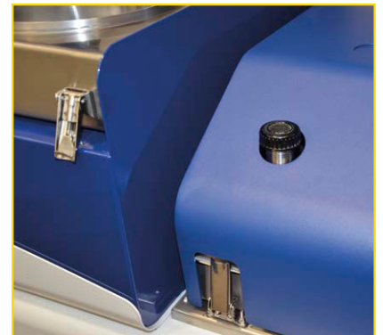
Possibility of introducing the solvent with a foot-pump or directly from a pipe placed over the distillation chamber cover.
