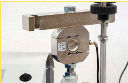
Possibility to place load cells with different capacities, in addition to 10 kN standard cell.
