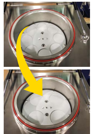
Double-face sample holder for testing up to 4 samples Ø 70 x 45 mm, or 8 samples Ø 55 x 35 mm
