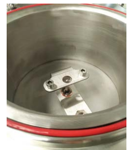
Platinum RTD probe for measuring the test temperature placed at the sample level.
