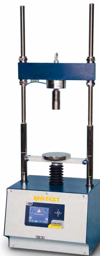
S205-05N with load cell
