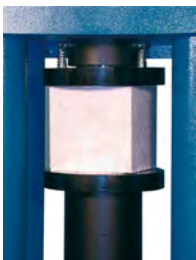
Compression on concrete
