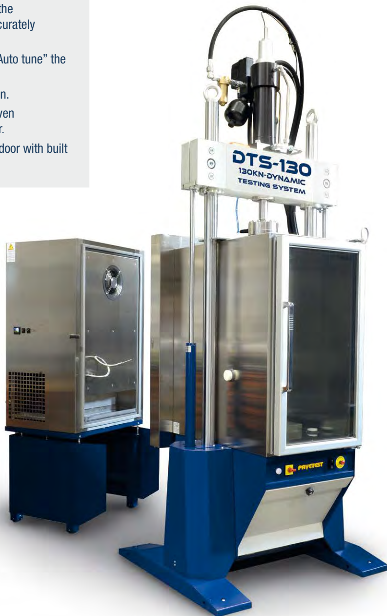
Two piece temperature controlled cabinet
