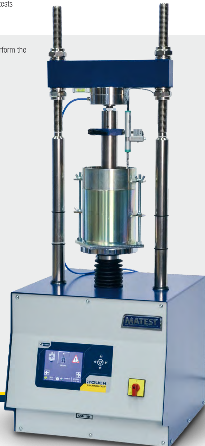
S215A with CBR mould
