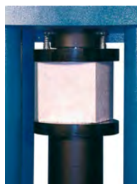
Compression on concrete
