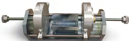
B282-08 TSRST specimen gluing jig (needed accessory)
