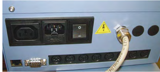
RS232 for PC connection only upon customer request LAN connection to internet
