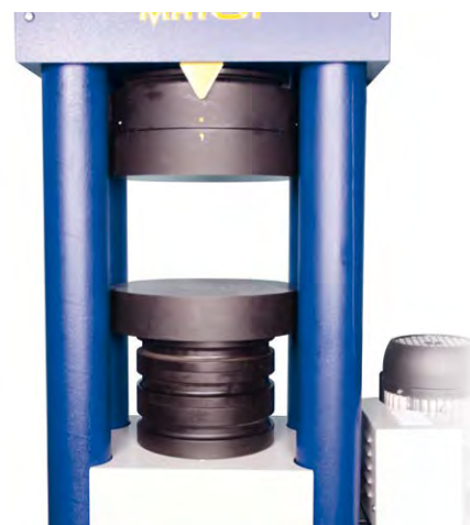
C089-02N with standard lower plate Ø 287 mm (weight 30.3 kg)
