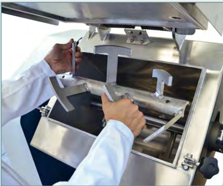
B026-05N Detail of the detachable mixing shaft
