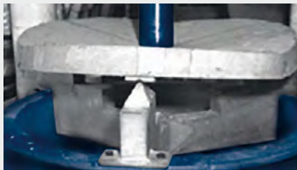
Test on RDP and Load-deflection curve according to ASTM C1550
