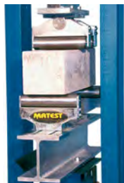
Flexure on concrete
