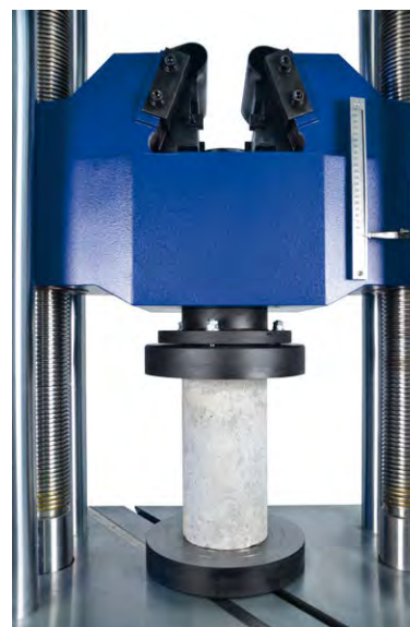
H001C-50 Detail of the standard compression platens
