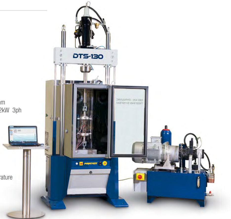
B240 130 kN Servo-Hydraulic Dynamic Testing System with H009-01EN complete PC, B231 Temperature controlled cabinet, B240-03 Exchanger oil/water, HPS (hydraulic power supply)
