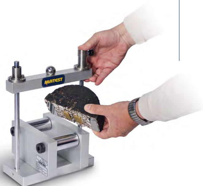
Asphalt specimen positioning
