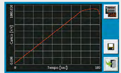
Automatic pace rate up to failure to avoid specimen's crumbling according to ASTM C39 Specification.
