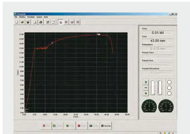
Tensile test on a steel specimen without extensometer; it displays the yield point with the possibility of increasing the dimensions of the graph area by means of the zoom function.
