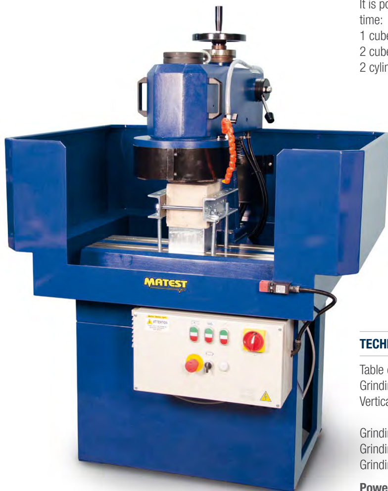
C299 with C300-06N holding one 150 mm cube
