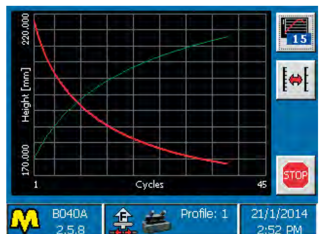
Height-Cycles and Density-Cycles curves during compaction
