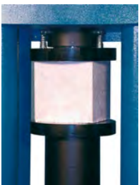
Compression on concrete
