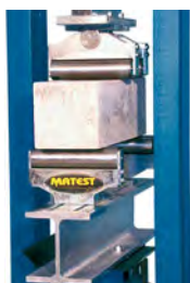
Flexure on concrete
