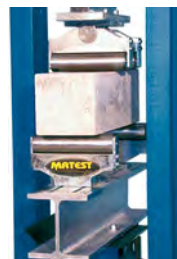
Flexure on concrete
