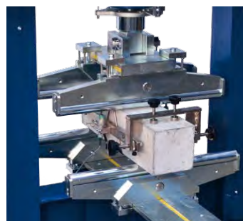
C090-15 + C109-15N fixed on the flexural machine C090-07N
