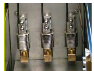
Detail: 3 load cells 500 N
