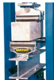
Flexure on concrete
