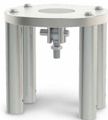
B260-10 Pull off tension jig
