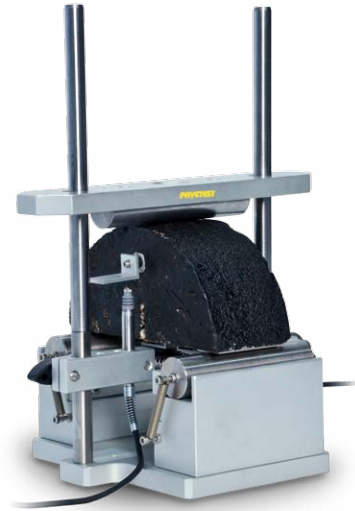
B254-02 KIT AASHTO TP124 | ASTM D8044 SCB testing kit
