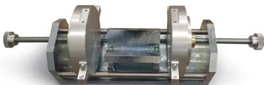
B282-08 TSRST specimen gluing jig (needed accessory)
